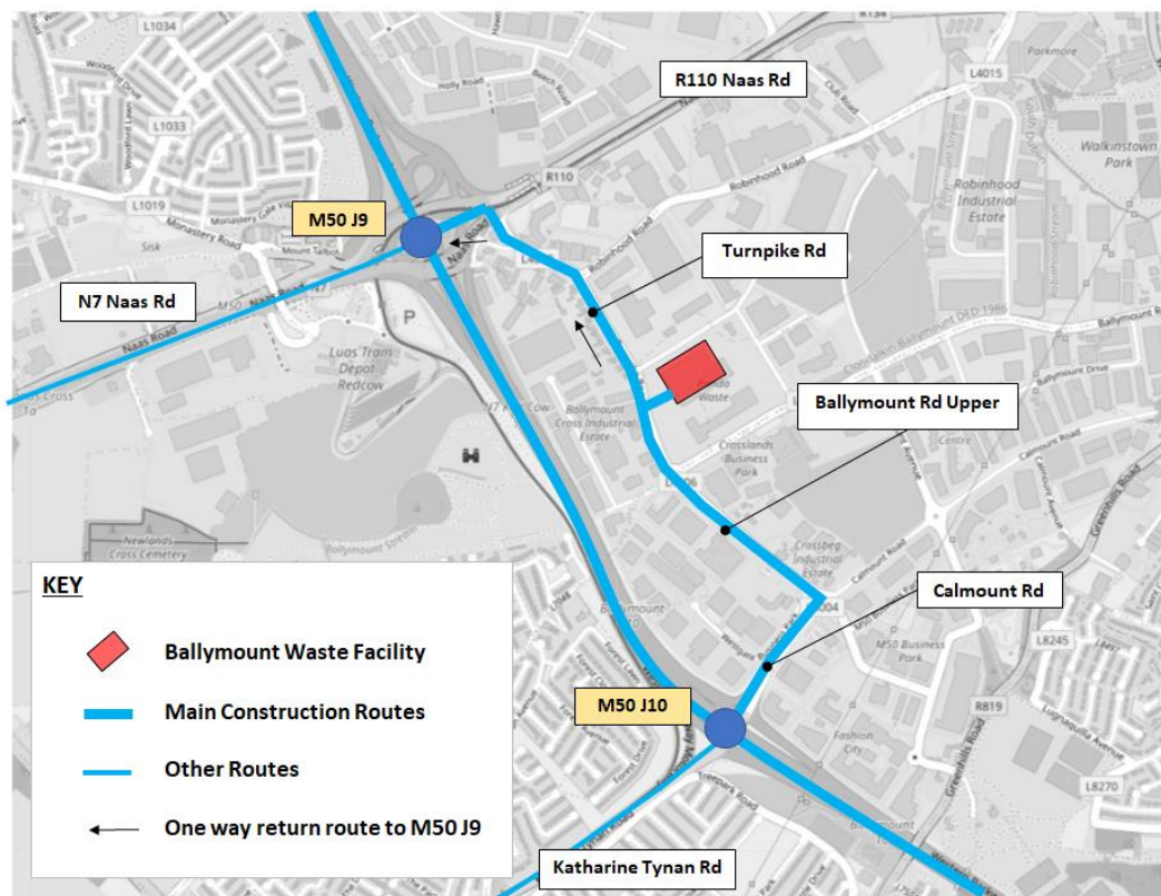
Figure 1. Proposed HGV routes during construction
