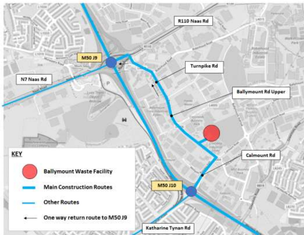
Figure 14.3: Suggested Construction Traffic Routes (Source Google Maps / SYSTRA annotations)
